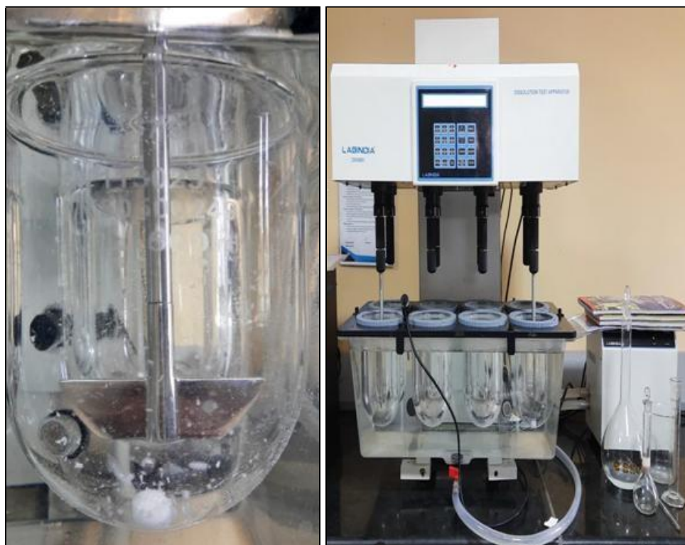
FIG. 1: TYPICAL DISSOLUTION TEST OF TABLETS OF METFORMIN HCl
